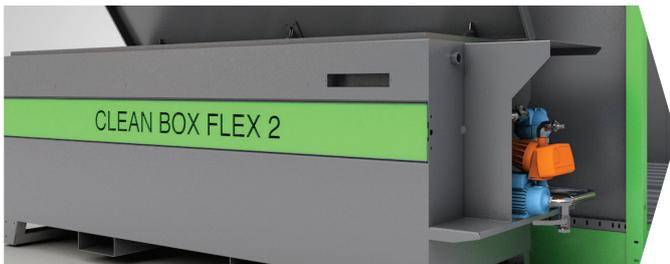
Water is pumped into this tank from the rear collection tank. This tank contains additional filters.
