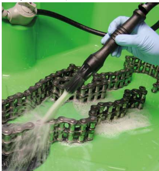
Cleaning oil-contaminated parts in the BIO-CIRCLE GT-i
